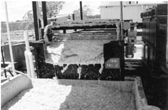
Collection of sludge from the electrocoagulation treatment of stick water at Burrangong Meat Processors
